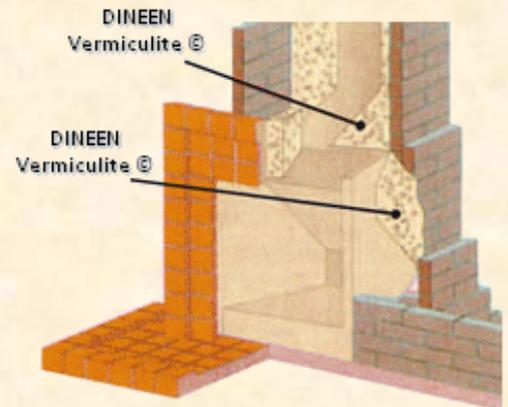
**DINEEN** vermiculite is manufactured at our own works in Ireland and is suitable for insulating chimney liners, backfill for firebacks and boilers, pipe insulation, roof and floor insulation, thermal & acoustic insulation and much more.
